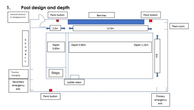
The dimensions of the pool are: small pool  $6m \times 2.5m$  and main pool  $12.5m \times 6m$  and it contains  $86.64m^3$  of water. The depth at the shallow end is: small pool 0.65m and main pool 0.9m and at the deep end small 0.65m and main 1.15m. Emergency exits are indicated on the plan above.
